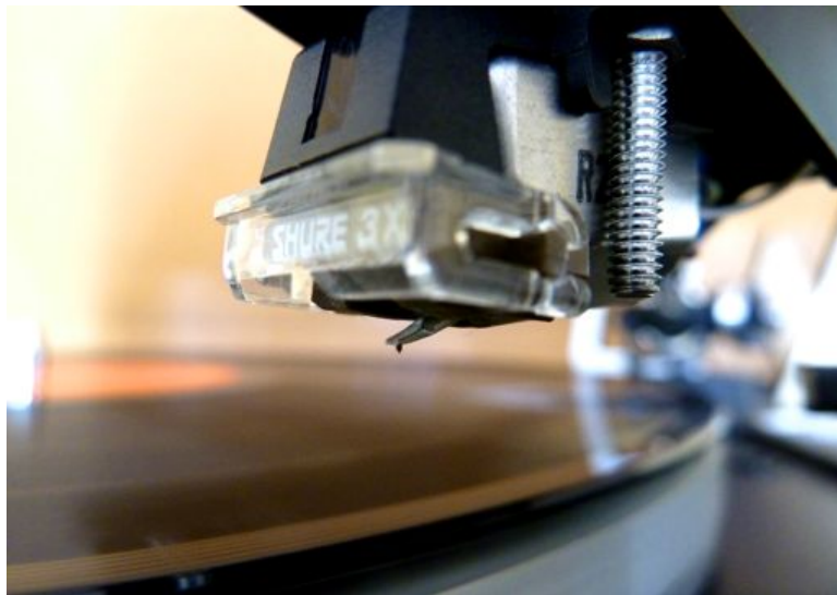
Figure 1.6: Turntable stylus used to read audio track on records. Photo credit: Ben Topple
